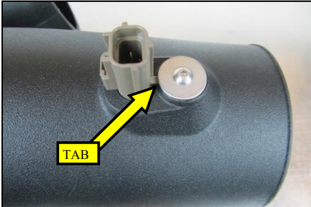
14. Gently insert the Air Temp Sensor into the Airaid Intake Tube as shown, with the locating tab inside of the slot in the sensor boss. Secure the sensor using The remaining 8-32 Screw and #8 Fender Washer
