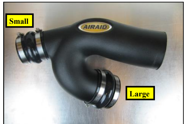
15. Slide the Hump Hoses and Clamps onto the Airaid Intake tube as shown. The Small Hump Hose will use the #48 Clamps and the Large Hump Hose is to use the #64 Clamps. Apply the Airaid Decal onto the Tube as shown.
