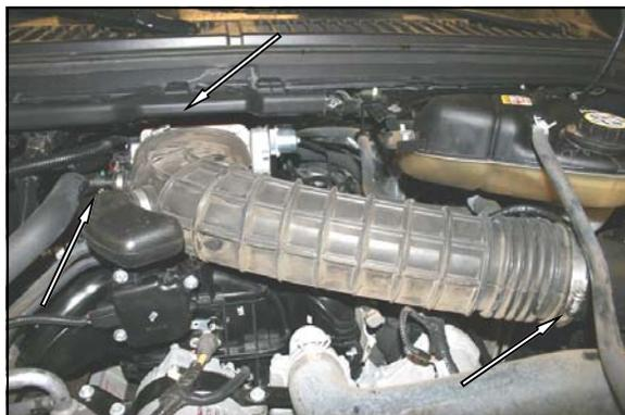
5. Reinstall the factory intake tube onto the throttle body, and then onto the factory air cleaner cover. Tighten the two hose clamps, and reconnect the breather hose.
