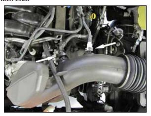
2. Disconnect the EVAP and crank case vent quick disconnect fittings.
