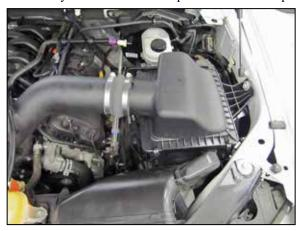
8. Install the AIRAID® intake tube into the coupler at the air filter housing and then into the coupler at the throttle body, adjust the tube for best fit and then secure with the provided hose clamps.
