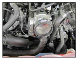
7. Install the provided coupler hose (08615) onto the throttle body and secure with the provided hose clamp.
