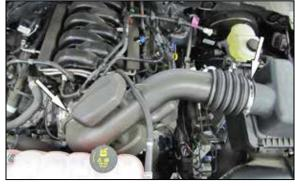
3. Loosen the hose clamps that secure the factory intake tube to the air filter housing and throttle body and then remove the intake tube from the vehicle.
