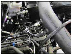
9. Connect the EVAP and crank case vent lines to the quick connect fittings installed into the AIRAID® intake tube.
