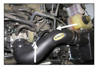
**10.** Reconnect the breather lines to the Airaid Intake Tube.
