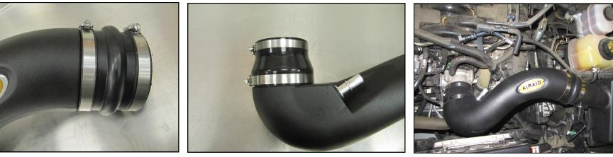
7. Install the hump hose (#3) and two #60 hose clamps (#9) onto the Intake Tube as shown. Leave the hose Clamps loose for now.
