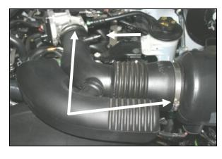
**3.** Slide the green tab on the factory breather hose, and remove it from the factory intake tube. Using a 5/16" socket, loosen the hose clamps on each end of the factory intake tube and remove it from the engine.
