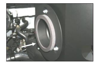
7. Install the gasket (#16) onto the filter adapter.
