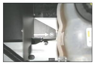
**12.** Align the hole in the **CAD** with the hole in the factory coolant reservoir mount. Insert one M6-1x25 hex bolt (#18) and 1/4" flat washer (#13) through the hole in the **CAD**, through the coolant reservoir mount, and into the speed nut below it.
