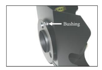
**6.** Insert three ½-20 x 7/8" bolts (#12), and ½" flat washers (#13) through the **CAD**. Place one bushing (#14) at each hole between the **CAD** and the filter adapter (#5). Next, secure the assembly using three ½" flat washers (#13), and ½-20 locknuts (#15).
