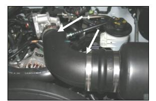
15. Install the reducer coupler (#7) onto the Airaid Intake Tube (#4) using one #48 hose clamp (#23) on the small end of the coupler, and one #52 hose clamp (#24) on the big end. Slide the tube into the hump hose first, and then over the throttle body. Adjust for fit, and tighten the clamps. Reconnect the factory breather hose.
