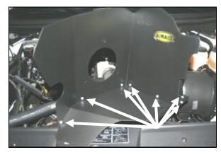
**5.** Assemble the Airaid Cool Air Dam (CAD) panels (#2, #3) using seven 6-32 x 5/16" screws (#9), #6 flat washers (#10), and 6-32 keps nuts (#11).
