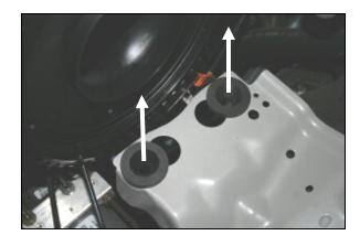
**9.** Remove the two factory grommets from the factory airbox mounting plate.
