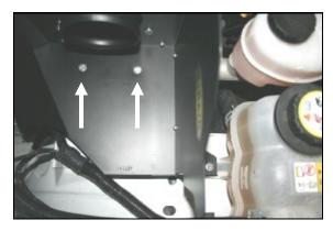
13. Insert two  $\frac{1}{4}$  - 20 x 7/8" bolts (#12) and  $\frac{1}{4}$ " flat washers (#13) through the holes in the **CAD** and thru the grommets. On the underside of the factory airbox mounting plate, align the long/narrow bracket (#19), two  $\frac{1}{4}$ " flat washers (#13), and two  $\frac{1}{4}$  - 20 locknuts (#15) with the  $\frac{1}{4}$ -20 x 7/8" bolts. Tighten the assembly securely.
