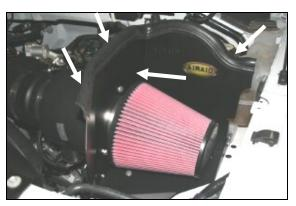
**16.** Install the Airaid Premium Filter (#1) onto the **CAD** and tighten the clamp. Install the weather strip (#8) onto the top edge of the **CAD** as shown. (Hint: start at one end and work your way around to the other.)
