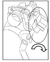
15. <u>4.6L engines</u>: Rotate the resonator box 90 degrees to provide clearance for the 3/4 x 12" Lhose (#7). Install the 3/4"x12" L-hose (#10) onto the Airaid Intake tube and the resonator box and secure it using the two #22 speed clamps (#23).
