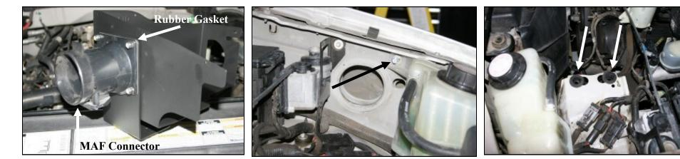
7. Attach the MAF bracket (#6), rubber gasket (#18), and factory MAF sensor housing to the Cold Air Dam (CAD) using four 1/4-20x7/8" hex bolts (#15), and 1/4" Nylock nuts (#17), as shown. Make sure that the MAF sensor connector is on the bottom when assembly is complete. Refer to the line drawing above for reference.
