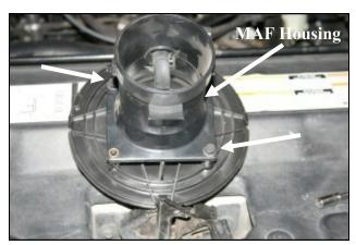
**5.** Remove the bolts that secure the MAF sensor housing to the adapter. Separate the adapter plate from the MAF sensor housing and save the sensor and housing for reinstellation in step #7
