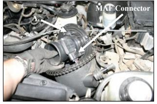
4.Unlatch the clamp on the canister to separate the two halves. Once separated, remove the factory air filter.A) Next, slide the large round plastic Mass Air Flow (MAE) sensor adapter plate from the canister. To do
