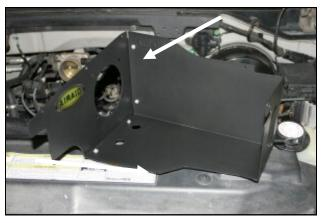
**6.** Assemble the MAF panel (#3), and bottom panel (#4) as shown using four 6-32 screws (#12), four flat washers (#13), and four Kep nuts (#14) as shown.
