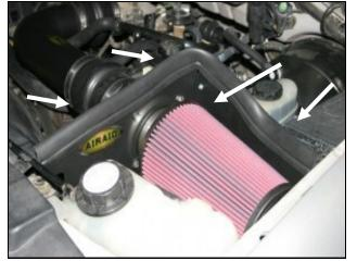
16. Reinstall the beauty cover using the 3 factory bolts. Install the Airaid Premium Filter (#1) as shown, and tighten the hose clamp.
