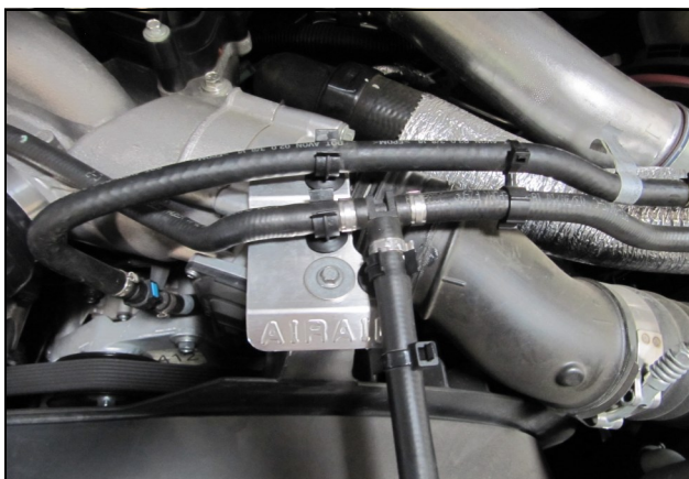
16. Mount the Hose Bracket as shown, using the factory bolt removed in step 6. . Secure the coolant lines in the Hose Anchors.
