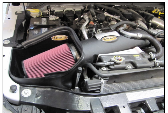
18. Install the Airaid Premium Filter (#1) inside the CAB and complete the install by trimming the CAB with the Weather Strip (#6).
