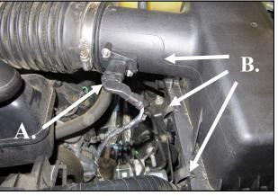
**2. A.** Disconnect the Air meter in the factory airbox top.
