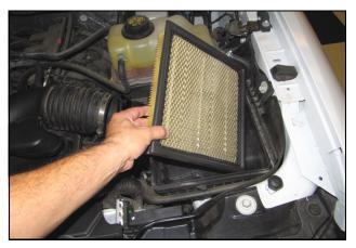
4. Remove the Factory air filter.
