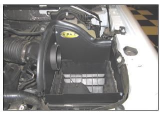
**12.** Install the Weather Strip (#5) to the Panel assembly as shown, with the contour rolling away from the filter area.
