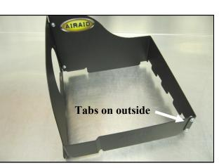
**5.** Assemble the Front and Rear Panels (# 3 & #4) as shown with the tabs on the outside of the assembly.
