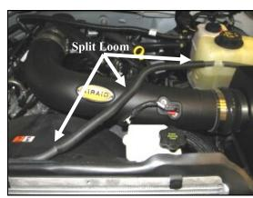
9. A.) Insert the Airaid Intake Tube into the couplers as shown. Check for alignment, and tighten all
