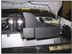
**5. A.)** Install the Silicone Hump Hose (#6) and two #64 Hose Clamps(#14) onto the Quick Fit assembly. Leave the clamps loose for now.
