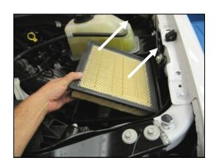
**3.** Remove the factory air filter from the lower half of the airbox.
