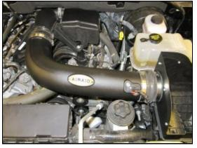
8. A.) Insert the Airaid Intake Tube into the couplers as shown. Check for alignment, and tighten all clamps.
