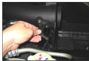
9. Re connect the Mass Air Flow Sensor.
