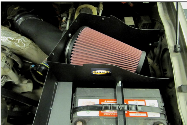
16. Install The Airaid Premium Filter (#1).
