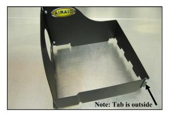
4. Assemble the two Quick Fit Panels (#4 & #5) as shown using four 6-32 screws (#12), flat washers (#13), and Kep Nuts (#14). The panel tabs are to be on
