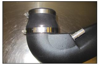
9. Install the Silicone Reducer (#7) and Hose clamps onto the Airaid Intake Tube (#2). Place the #56 clamp (#15) on the Throttle body side of the reducer, and the #64 clamp (#17) on to the tube side.
