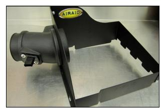
6. Transfer the MAF sensor into the Airaid Intake Tube and secure using two 8-32 x 1/2" button head screws (#10). Do Not Use The Factory Torx Head Screws.
