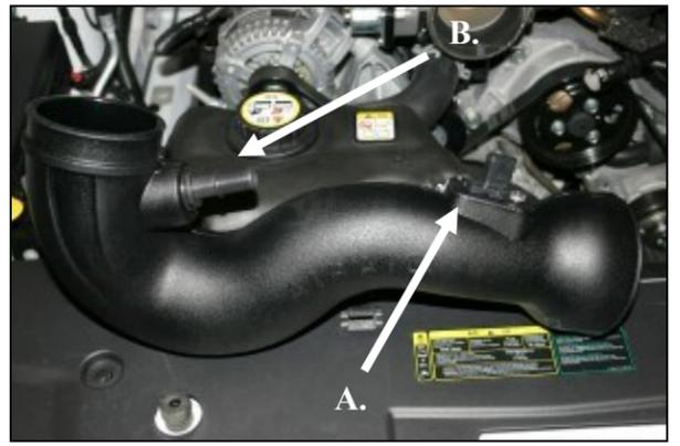
12. A.) Install the MAF sensor removed in step #5, into the Airaid Intake Tube (#2). Use the two supplied 8-32 button head bolts (#10), to securely fasten the MAF sensor. **Do Not Use The Factory Screws!** B.) Install the provided grommet (#16) into the intake tube and then install the factory fitting removed in step #5 into the grommet as shown.
