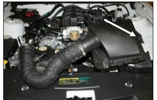
3. Remove the complete intake system as an assembly. Remove the factory grommet, and steel sleeve from the factory airbox for reuse in step #8.
