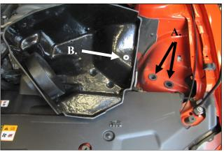
9. Transfer the factory air box mounting grommets. A) Locate and remove the Two Lower air box mounting grommets, and install them in the inner fender. B) Remove the Upper air box mounting grommet and steel sleeve, and re-install into the Airaid CAB.
