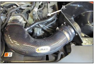
12. Install the Airaid Intake Tube into the couplers as
