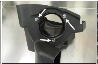
head bolts (#9), and Fat Washers (#8) into the Airaid Cool Air Box (CAB) (#3) as shown.
