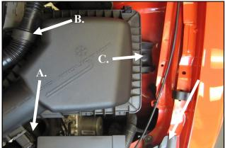
3. A) Disconnect the wiring harness from the Mass Air Flow sensor (MAF). Carefully pry the harness anchor from the air box using a screwdriver. B) Separate the resonator tube from the Air box lid. C) Using a 10mm socket, remove the bolt securing the air box to the inner fender and remove the air box assembly. This bolt will be reused in step 10.
