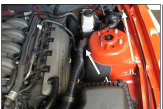
**4.** Remove the resonator assembly from the vehicle.
