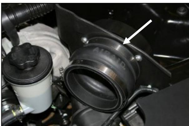
7. Install the provided hump hose (#4) onto the filter adapter using two #72 hose clamps (#15) as shown. Leave the two hose clamps loose for now.
