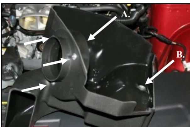
4. A.) Install the filter adapter (#7) using three 1/4-20 button head bolts (#11), and flat washers (#10) into the Airaid Cool Air Box (CAB) (#3) as shown. B.) Reinstall the small grommet and sleeve (removed in step #3) into the hole in the CAB.
