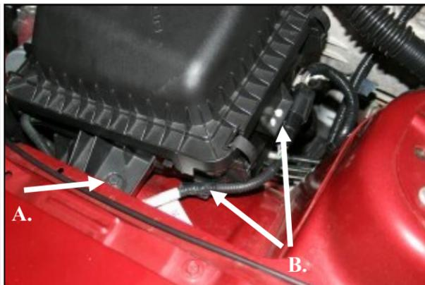
2.A.) Using a 10mm socket, remove and save the bolt that secures the airbox to the fender.
