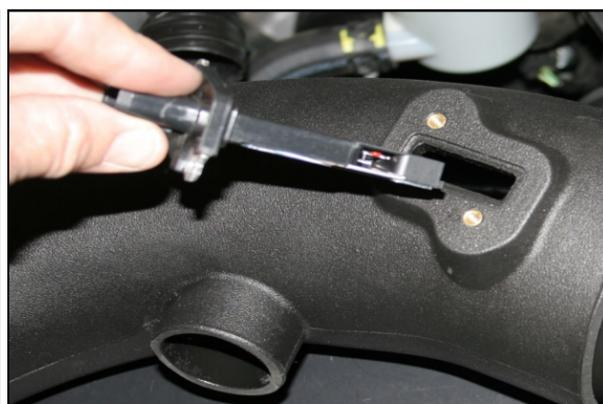
8. Install the MAF sensor into the intake tube using two provided 8-32x3/8" screws (#12).
