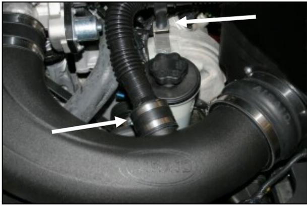
13. Install the air intake tube into the hump hose first, and then onto the throttlebody. Adjust for fit and then tighten all four hose clamps. Next, reinstall the factory resonator tube into the 1 3/4" coupler and tighten the hose clamp. Now "reset" the resonator tube onto the bracket.
