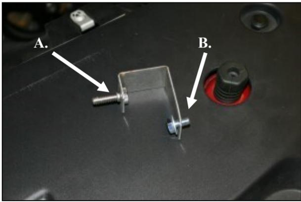
10.A.) Thread the 1/4-20 hex bolt (#13) into the resonator bracket (#21) and tighten as shown.
