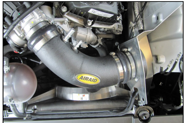
15. Install the Airaid Tube into the Hump Hose and Reducer as shown. Tighten all four Hose Clamps at this time.
