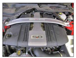
22. Reinstall the engine cover and strut tower brace and secure with the factory hardware.
