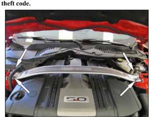
2. Remove the four nuts that secure the strut tower brace and then remove the strut tower brace from the vehicle.
