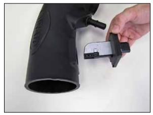
14. Install the mass air sensor assembly into the AIRAID® intake tube as shown and secure with the provided hardware.
