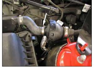
6. Release the clamp that secures the sound tube to the sound drum and then disconnect the sound tube from the drum. Remove the factory intake tube assembly from the vehicle
