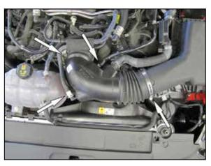
5. Disconnect the two vent lines attached to the factory intake tube, loosen the hose clamps that secure the intake tube to the throttle body and air filter housing.
