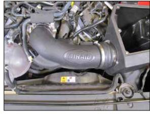
18. Install the AIRAID® intake tube into the coupler at the filter adapter and then into the coupler at the throttle body, adjust the tube for best fit and then secure with the provided hose clamps.
