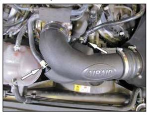
19. Connect the EVAP and crankcase vent lines to the fittings installed into the AIRAID® intake tube.
