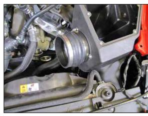
17. Install the provided hump coupler onto the filter adapter and secure with the provided hose clamp.
