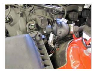
7. Install the provided cap onto the sound drum as shown
