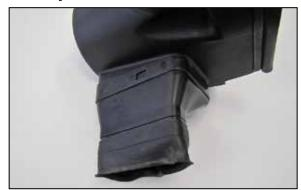
10. Remove the fresh air intake duct from the factory air filter housing and install it onto the AIRAID<sup>®</sup> air filter housing.
