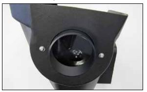
6. Install the provided filter adapter into the AIRAID<sup>®</sup> filter housing and secure with the provided hardware.
