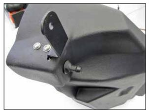
7. Install the mounting bracket and mounting stud onto the air filter housing using the provided hardware.
