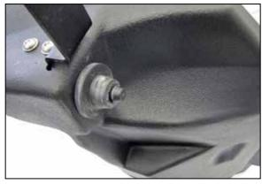
8. Install the factory air box mounting bracket onto the mounting stud installed onto the AIRAID<sup>®</sup> air filter housing in the previous step.
