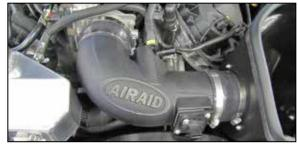
17. Install the AIRAID<sup>®</sup> intake tube into the coupler at the heat shield and then the throttle body, adjust the tube for best fit and then secure with the provided hose clamps.
