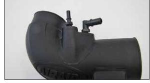
15. Install the provided vent fittings into the AIRAID<sup>®</sup> intake tube as shown. NOTE: Plastic NPT fittings are easy to cross thread. Install the vent fitting "hand" tight, then turn it two complete turns with a wrench.
