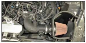
19. Connect the factory vent lines to the fittings installed into the AIRAID $^{\circ}$  intake tube.
