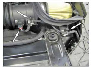
2. Disconnect the mass air sensor electrical connection and then unhook the harness retaining clips.
