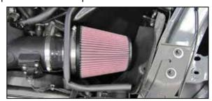
18. Install the AIRAID<sup>®</sup> air filter onto the filter adapter and secure with the provided hose clamp. Reconnect the mass air sensor electrical connection.
