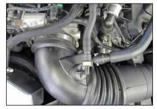
4. Loosen the hose clamp at the throttle body. Disconnect the vent lines attached to the intake tube and then remove the intake tube from the vehicle.
