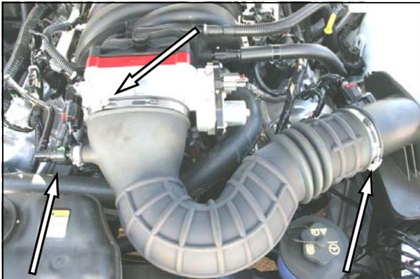
5. Reinstall the intake tube, and tighten the hose clamps. Reconnect the breather hose to the intake tube.
