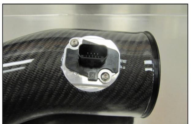
6. Using the supplied Torx bit, (#19) remove the MAF sensor from the factory airbox and transfer it into the Airaid Tube assembly (#2). Install the MAF sensor using two provided 8-32x3/8" screws (#10).
