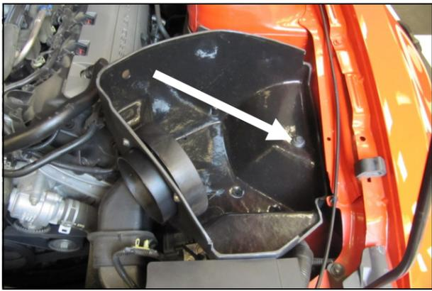
**10.** Install the CAB into the vehicle. Make sure that the Air inlet of the CAB aligns with the factory duct, and the two locating pins on the bottom align with the factory grommets. Next reinstall the factory bolt that was removed in step #3 through the steel sleeve and grommet and into the inner fender.
