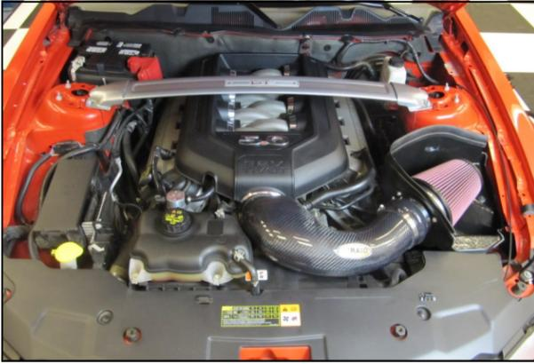
**14.** Replace the engine cover and shock tower brace.
