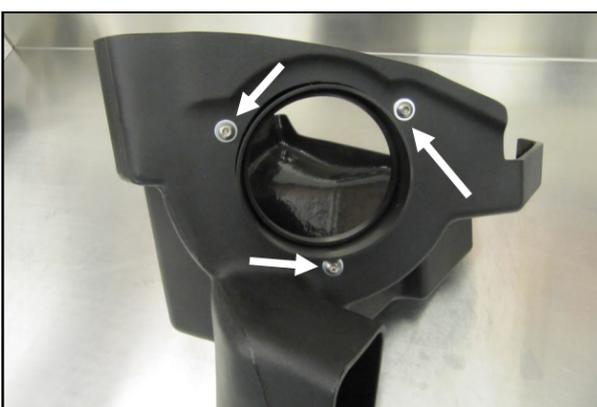
8. Install the filter adapter (#4) using three 1/4-20 button head bolts (#9), and Flat Washers (#8) into the Airaid Cool Air Box (CAB) (#3) as shown.
