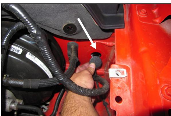
5. Insert the Fire Wall Plug (#16) into the resonator hole.
