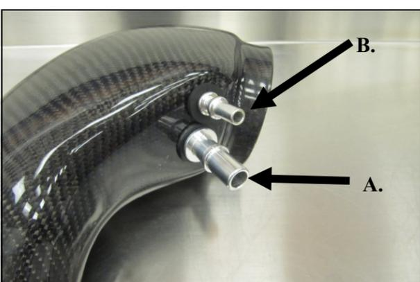
7. Install the Grommets and Fittings into the Airaid Intake Tube (#2): **A)** All models will require the use of the 5/8" Fitting (#15) and the 5/8" Grommet (#12). **B)** Automatic transmission equipped vehicles will also use the 3/8" Fitting (#14) and 3/8" Grommet (#11). Manual transmission vehicles will not need the 3/8" components and will use the Blind Grommet (#13)
