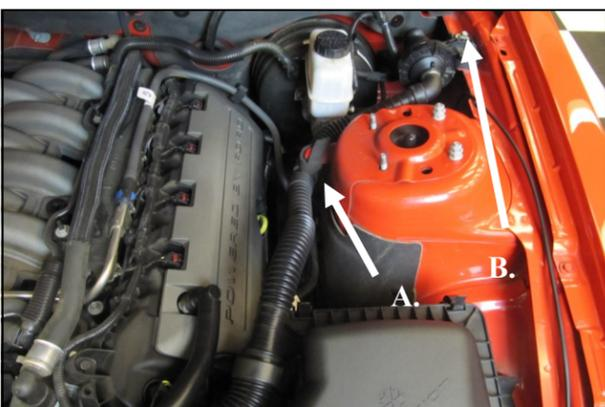
4. Remove the resonator assembly from the vehicle. **A)** Slide the hanger off of the strut tower tab. **B)** Remove the 6mm bolt securing the diaphragm body to the inner fender. Slide the resonator tubing out of the firewall and set the assembly aside. It will not be reused.
