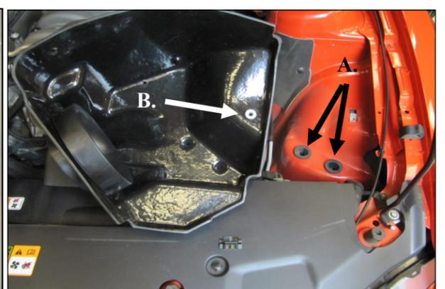
9. Transfer the factory air box mounting grommets. **A)** Locate and remove the Two Lower air box mounting grommets, and install them in the inner fender. **B)** Remove the Upper air box mounting grommet and steel sleeve, and re-install into the Airaid CAB.
