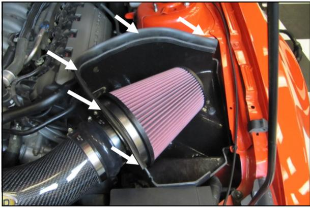
**13.** Install the Airaid Premium Filter (#1) onto the Filter Adapter and tighten the hose clamp. Install the Weather Strip (#7) onto the CAB with the contoured edge going away from the filter. Start at the front of the vehicle and work your way back.
