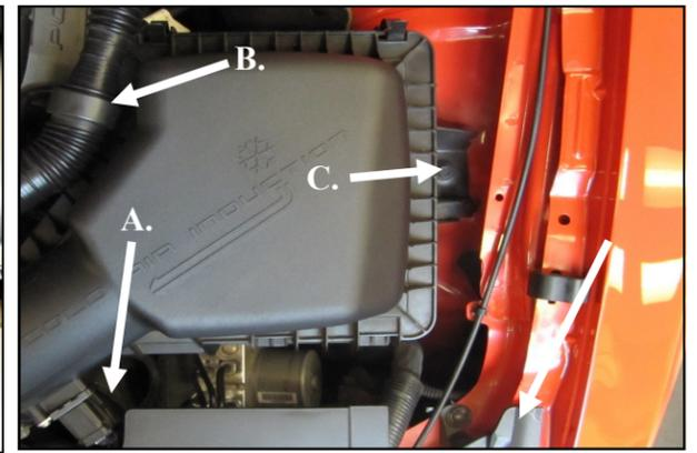
3. **A)** Disconnect the wiring harness from the Mass Air Flow sensor (MAF). Carefully pry the harness anchor from the air box using a screwdriver. **B)** Separate the resonator tube from the Air box lid. **C)** Using a 10mm socket, remove the bolt securing the air box to the inner fender and remove the air box assembly. This bolt will be reused in step 10.
