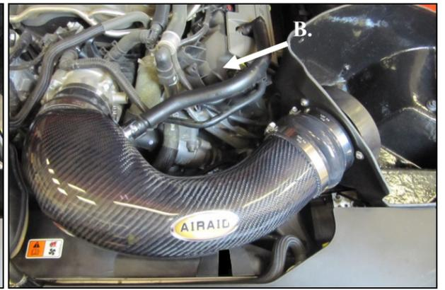
**12.** Install the Airaid Intake Tube into the couplers as shown, and tighten all Hose clamps. Reconnect the breather line/lines to the Aluminum Fittings depending on your application. Reconnect the Mass Air Flow sensor, which is now located in the lower back side of the intake. Slide the locking tab back into the connector
