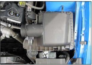
**8.** Unclip the factory air box lid and slide it off of the tabs in front. If you are installing an Airaid Jr. kit, install the Airaid Premium filter at this time. Leave the air box lid unattached for now.
