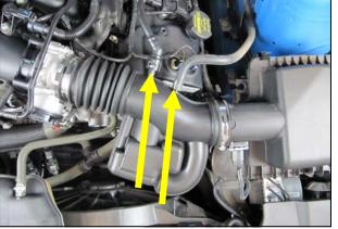
2. Carefully depress the connector lock tabs, and disconnect the crank case breather line and the brake aspirator line if equipped, (AT models only).
