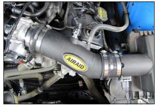
**10.** Slide the air box outlet into the Coupler. Connect the breather lines from step 2 to the Airaid Intake Tube. Rotate the tube if necessary to clear the Hood and valve cover and tighten all Clamps.
