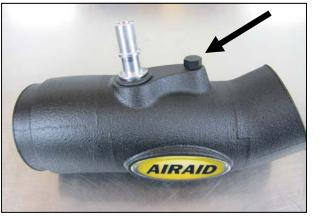
5. Manual transmission vehicles will not need the Barbed Fitting and will use the Threaded Plug.
