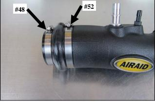
6. Slide the Hump Hose, one #48 Clamp, and one #52 Clamp onto the Intake Tube as shown. Do not tighten the Clamps at this time.
