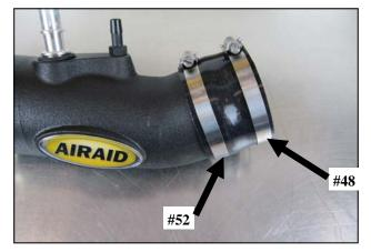
**7.** Slide the Reducer, one #48 Clamp, and one #52 Clamp onto the other side of the Intake Tube as shown. Do not tighten the Clamps at this time.
