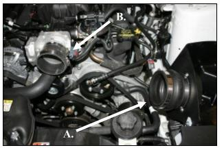
11. A.) Install the hump hose (#4) onto the filter adapter as shown using two #72 hose clamps (#13). Leave the clamps loose for now. B.) Install the supplied reducing coupler onto the throttlebody as shown using one #48 hose clamp (#11), and one #52 hose clamp (#12). Tighten only the hose clamp on the throttlebody at this time.
