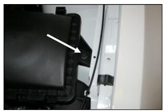
**2.** Remove the bolt that holds the factory airbox to the driver's side inner fender. (Save this bolt for later use in step #9).
