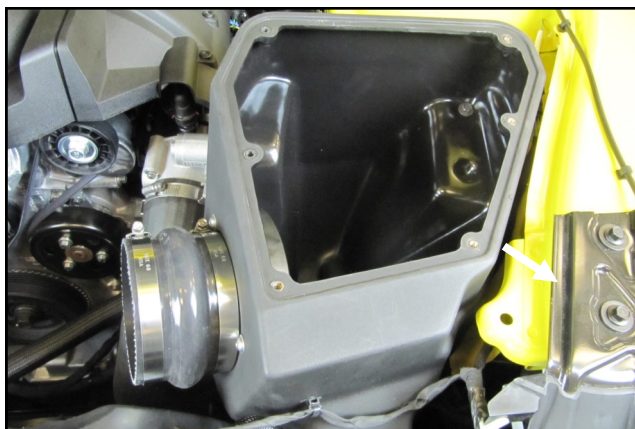
14. Slide the Hump Hose and Clamps onto the Filter Adapter as shown. Do not tighten the clamps at this time.
