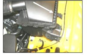
**2.** Remove bolt that holds the factory airbox to the fender. (Save bolt for later use in step #7).
