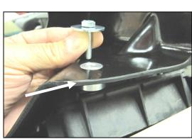
**8.** Slide the Aluminum Spacer (#17) underneath the **CAD** and into the hole as shown. Secure the CAD to the inner fender using the OEM bolt from step # **2** and the supplied 1/4" Fender Washer (#18).
