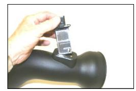
**12.** Install the MAF sensor from step #5 into the Airaid Intake Tube. Use the two supplied 8 -32 button head bolts (#10), to securely fasten the MAF sensor.
