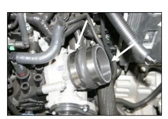
7. Install the supplied hump hose (#6), and two #44 hose clamps (#16) onto the throttlebody as shown. Tighten only the clamp on the throttlebody.
