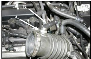
**3.** Remove the factory flexible intake tube from the vehicle. Remove the Oeticker clamp, and then remove the large plastic elbow from the flexible intake tube. It will be reused in step #12.
