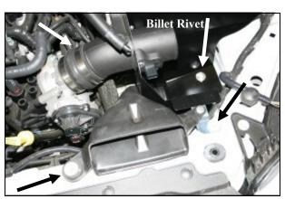
14. Install the CAD into the vehicle making sure to slip the intake tube into the hump hose as you lower the assembly into place. After you have the intake tube correctly located into the hump hose, insert the billet rivet (#19) thru the CAD and into the factory grommet in the inner fender well. Tighten the hose clamp on the hump hose and then reinstall the two factory bolts removed in step #1 that secure the scoop to the radiator support. Reconnect the Mass Air Flow sensor!
