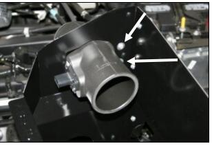
11. Now turn the intake tube counterclockwise until the mounting holes align thru the panel. Secure the tube to the panel using the two 1/4"-20 button head bolts (#10) and 1/4" washers (#11).
