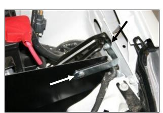
**15.** Install the side bracket (#17) onto the **CAD** as shown using the factory bolt removed in step #6, and one 1/4"-20x5/16 hex bolt (#13), two 1/4" flat washers (#12), and one lock nut (#14).
