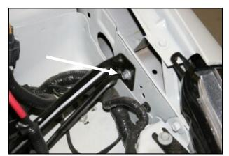
**6.** Remove one bolt that secures the brace to the inner fender. It will be reinstalled in step #15.
