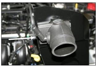
**12.** Insert the factory elbow removed in step #3 into the large grommet on the side of the intake tube as shown. A drop or two of dish soap or something similar will help make the elbow slide thru the grommet easier.
