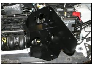
9. Auto Transmission vehicle only: Assemble the two Cool Air Dam panels (#3 & #4) using 7 screws (#8), washers (#9), and nuts (#10) as shown. Make sure that the bent flanges where the panels screw together, are on the outside of the box. Note: Use panel #3 with tag marked "AUTO".
