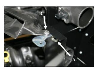
**13. A.)** Install the front bracket (#18) onto the front of the **CAD** as shown using one 1/4"-20x5/8" hex bolt (#13), two 1/4" flat washers (#12), and one lock nut (#14). **B.)** Next mount the factory scoop to the bracket as shown using one 1/4"-20x5/8" hex bolt (#13), two 1/4" flat washers (#12), and one lock nut
