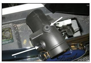
**8.** Install the small grommet (#20) into the hole on the top of the Airaid intake tube (#2). Now install the large grommet (#21) into the hole on the side of the tube.
