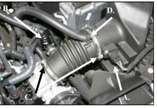
2. A.) Pull the red tab on the bottom, and then squeeze the Mass Air Flow sensor wiring connector and disconnect it from the sensor. B.) Push the tab, and disconnect the breather hose from the plastic elbow. C.) Loosen the two factory clamps on the flexible intake tube. D.) Remove the Oetiker clamp, and then carefully remove the small plastic elbow from the flexible intake tube leaving the breather hose connected to the elbow.
