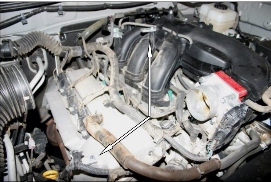
7. Install one 1" extension plate (#9) using a 6mm x 20mm bolt (#5) and flat washer (#4) on the valve cover with the long end of the spacer facing the right fender. Repeat this procedure on the top of the intake manifold at the location shown above.
