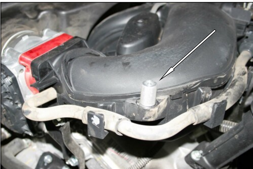
9. Install the 3/4" long round spacer (#11) on top of the threaded hole where the stud was removed on the intake manifold as shown and proceed to the next step.
