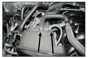
**2.** Disconnect the factory breather hose, and vacuum hose from the factory airbox lid.
