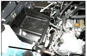
**4.** Using a 10mm socket, loosen the two bolts that hold the airbox base to the fender well, and
