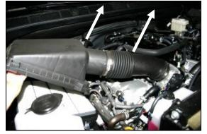
**3.** Unlatch the four metal clips that hold the airbox lid to the base and remove the intake tube and lid from the vehicle. Remove the factory air filter from the airbox base.
