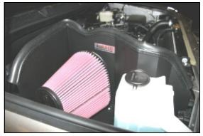
16. Install the Airaid Premium Filter (#1) onto the filter adapter and tighten the clamp. Next install the weather strip (#8) on top of the CAD as shown. For an easier install, start at the fender side of the CAD and work your way towards the radiator. Reinstall the factory beauty cover.
