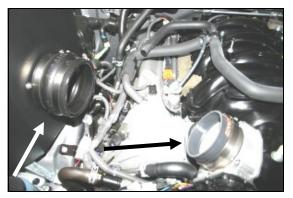
**10.** Install the hump hose (#6) with two #72 hose clamps (#19). Install the reducing coupler (#7) with the small end on the throttlebody. Install the #52 hose clamp (#17) over the throttlebody end. and the #56 hose clamp (#18) over the large end of the coupler. Leave the clamps loose for now.
