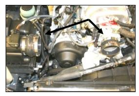
7. Install the hump hose (#3) onto the factory airbox, small end first, with two hose clamps (#6). Next install the reducing coupler (#4), small side first, onto the throttle body with two hose clamps (#7). Leave the clamps loose.
