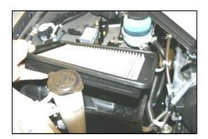
**6.** Remove the factory air filter, and install the Airaid Premium Filter (#1). Reinstall the factory airbox lid, and latch 4 clips.
