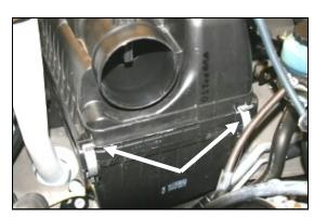
5. Unlatch the 4 clips on the factory airbox, and remove the lid.
