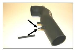
**8.** Install the 1/4" barb fitting (#10) into the Airaid Modular Intake Tube (#2) as shown. Now slide the 1/4"x4" hose (#8) onto the barb fitting.
