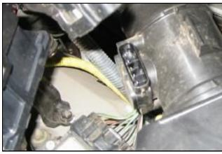
**3.** Disconnect the electrical connector from the Mass Air Sensor.
