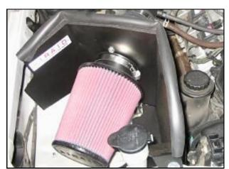
**15.** Mount the Airaid premium air filter inside the Cool Air Dam & press weather strip onto the top of the Cool Air Dam. (*Hint: start at a corner and work towards the ends*)
