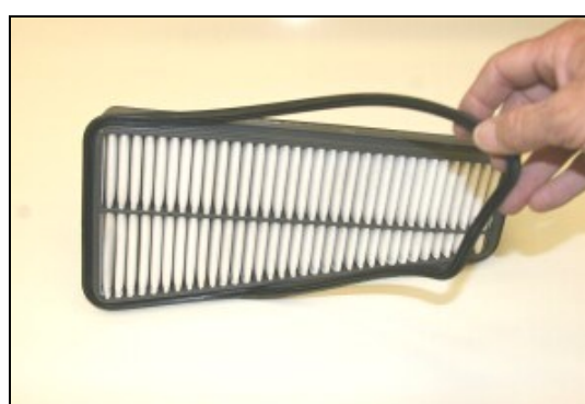
5. Remove the rubber gasket from around the factory air cleaner.
