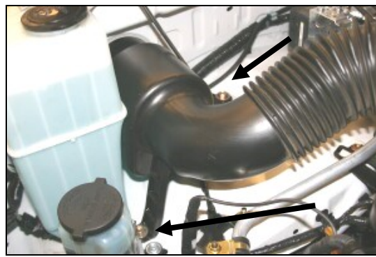
2. With a 12mm socket, remove two bolts that hold the intake tube to the fender.
