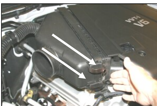
4. Unlatch the two clips that hold the cover on the factory airbox and remove the cover and the factory air cleaner.
