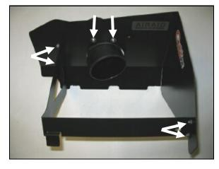
**5.** Assemble the Airaid Quick Fit Panels (#2, #3) using four 6-32 x 5/16" screws (#6), #6 flat washers (#7), and 6-32 keps nuts (#8). Next, install the air filter adapter (#4) using two  $\frac{1}{4}$ -20 x  $\frac{1}{2}$ " button head bolts (#9), and  $\frac{1}{4}$ " flat washers (#10).
