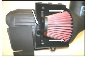
**6.** Carefully align the notch on the Airaid Premium Filter with the raised rectangle at the bottom of the factory airbox, then slide the air filter towards the elbow. Make sure the air filter is seated inside the factory housing securely, and replace the factory inspection cover, and tighten the screw.
