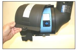
**2.** Remove the inspection cover to reveal the air filter.
