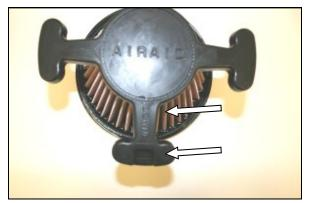
**4.** Locate the word "Down" on the filter and notice that there is a notch below it. It is important to locate this notch in the correct location in the bottom of the factory airbox.
