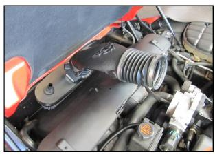
7. Reinstall the OEM intake tube onto the MAF and Filter Assembly then lower into the inner bumper area. When properly installed the Filter end cap will positively engage the grommet posts on the inner frame.
