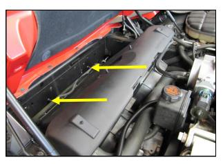
**6.** Inspect the inner bumper area and verify that none of the air box mounting grommets were retained during disassembly.
