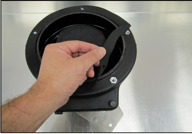
24. Place the Air Box Gasket (#22) onto the face of the Air Box and align the bolt holes.
