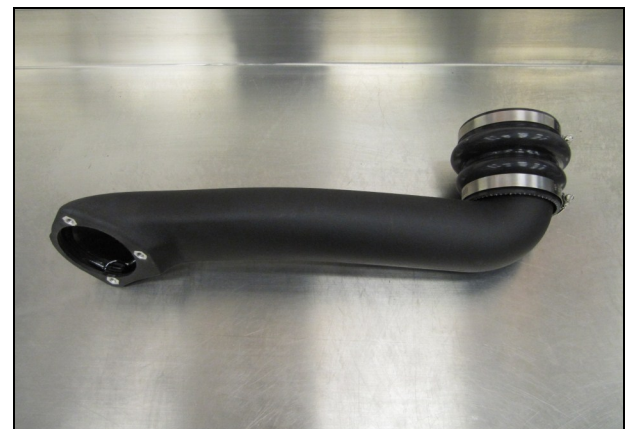
35. Slide the Hump Hose (#8) and clamps onto the Riser Tube (#4) as shown. The #52 Clamp (#19) is to be installed on the Tube side and the #60 Clamp (#20) on the other. Leave the clamps loose for now.
