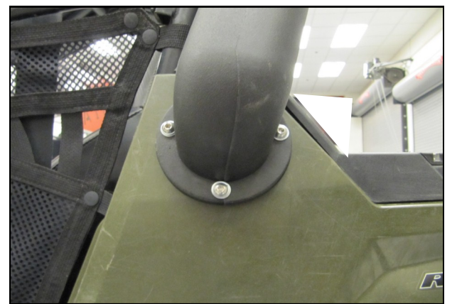
47. Replace the Threaded Studs, one at a time, with the remaining 1/4-20 x 1” Button Head Bolts and 1/4” Washers from the previous step. Make all three Bolts final tight.
