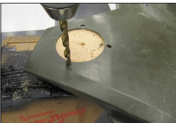
33. Drill 5/16" bolt holes in the panel.
