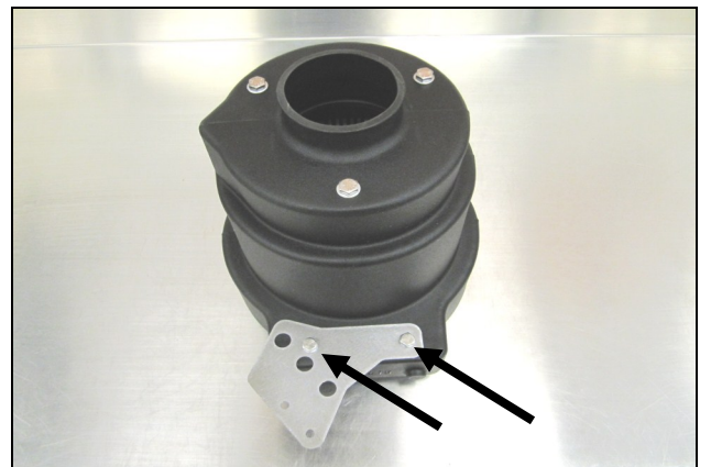
23. Mount the Transmission Bracket (#9) to the Air Box using two 1/4-20 x 5/8" Hex Bolts, and 1/4" Lock Washers (#15).
