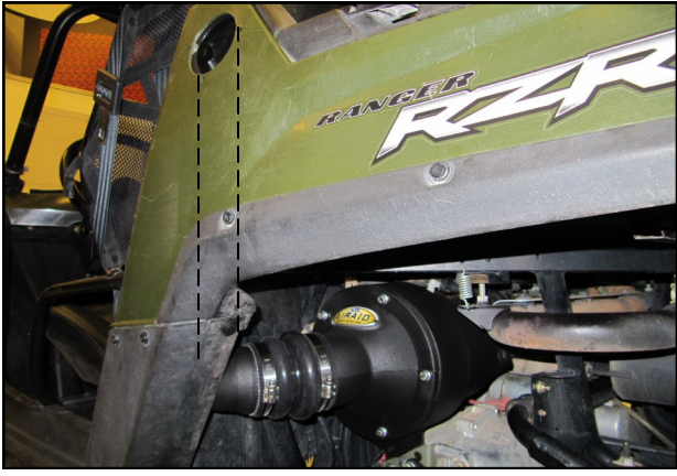
36. Position the Riser tube in the inner fender , behind the panel. Slide the Hump Hose and Clamps onto the Air Box inlet . Tighten both Hose Clamps.
