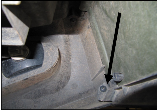
9. Underside view of fourth screw in need of removal.
