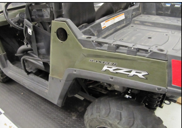
34. Reinstall the factory panels and the bed in the reverse order in which they were removed.
