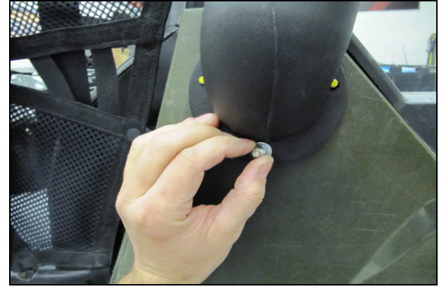
11. Mount the Snorkel tube on to the Threaded Studs and secure using one 1/4-20 x 1" Button Head Bolt (#2), 1/4" Lock Washer (#3), and 1/4" Flat Washer (#4). Do not fully tighten at this time.
