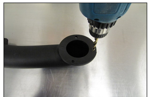
8. Remove the Gasket and drill the bolt holes in the Snorkel Flange. Start with 1/8" pilot holes and finish with 5/16" holes.
