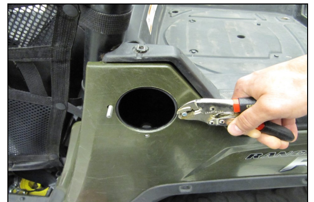
2. Using a pair of Locking Pliers, remove the Threaded Studs from the riser tube. Take care not to damage the threads for future installations.
