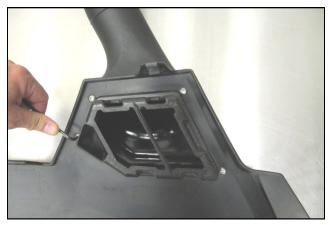
**8.** Attach the Fender Adapter to the outside of the factory Fender using four 1/4-20 button head screws (#13).
