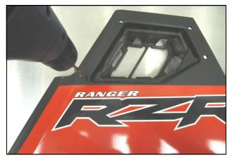
6. Using a 9/32" bit, drill out the pilot holes.
