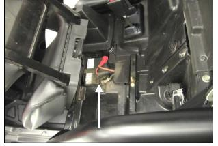
**1.** Place the range selector in Park and remove the seat from the vehicle. Disconnect the negative terminal on the battery.
