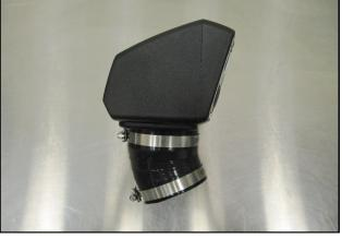
**13.** Install the Silicone Elbow (#6) and two #48 clamps onto the Inlet as shown. Leave the Hose Clamps loose for now.
