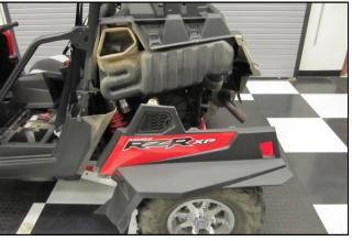
**2.** Remove the nine T-27 Torx head screws holding the fender in place. Remove the fender and place it on a work bench.
