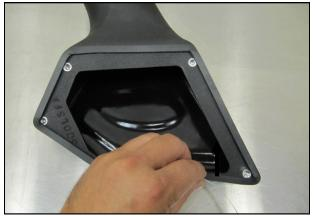
7. Prepare the mating surface of the Fender Adapter (#1) for the Foam Gasket Tape (#9) by cleaning with a prep solvent. Apply the gasket tape along the outside edge of the Fender Adapter as shown, avoiding the bolt holes.
