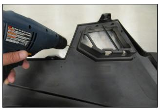
**5.** Using a drill and a 1/8" bit, drill out the four pilot holes in the inner fender.
