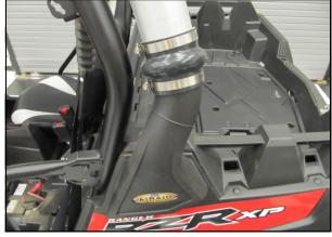
**12.** Install the Hump Hose (#7) and Aluminum Intake Tube (#2) onto the Fender adapter. Loosely install two #48 Clamps (#10) onto the Hump Hose.
