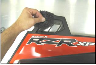
**3.** Remove the OEM filter cover and pre-filter from the fender and set aside. They will not be reused.
