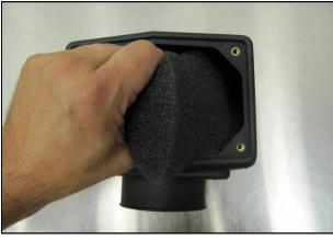
**10.** Insert the Foam Pre-Filter (#5) into the Snorkel Inlet (#3).
