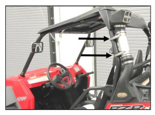
**15.** Secure the snorkel assembly to the roll cage using the Tube Mounts (#8) and #68 Clamps (#11).
