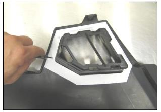
**4.** Cut out the paper Template. Align it with the edges of inner fender, and punch the four pilot holes. The Template is reversible and can be used on either side.
