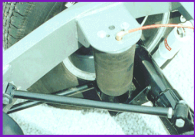
Rear suspension w/ 4 link and air ride
