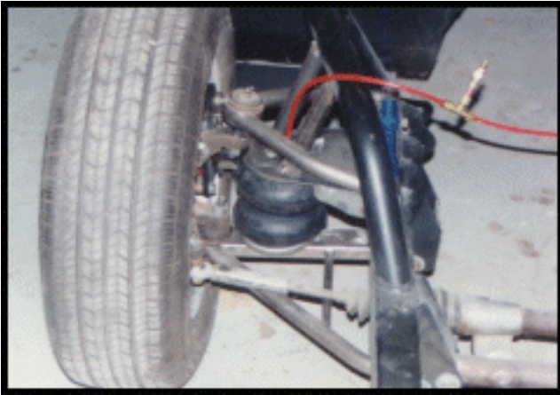
Aftermarket Mustang II installation [replaces coilover shock]
