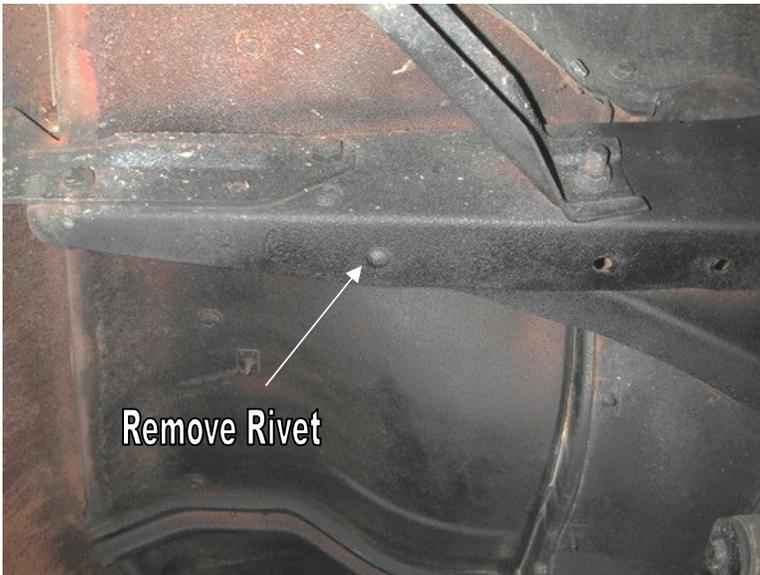
1. The sway bar frame plate will index off of this factory support brace rivet. Remove the rivet by grinding the head smooth, then drive it out with a hammer and punch.
