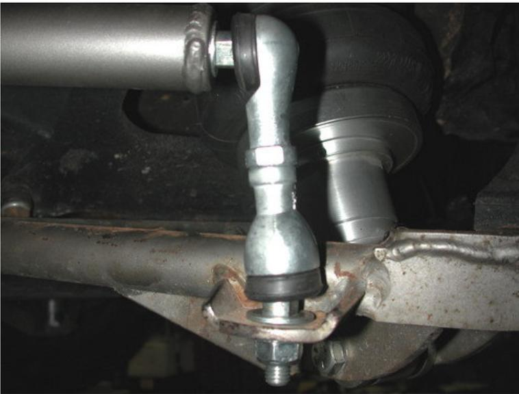
8. Bolt the 90 degree end of the PosiLink to the sway bar. A 3/8" flat washer and 12mm lock washer must be installed between the PosiLink and the bar.
