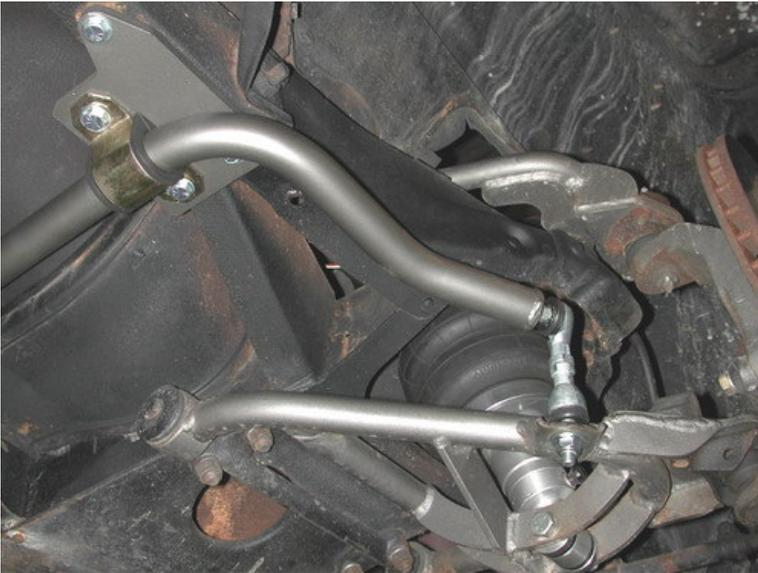
6. Apply lithium grease to the poly bushing. Install the bushing over the sway bar, and then place the bushing strap over the bushing.
