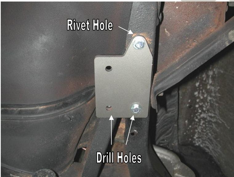
3. Using a 3/8" x 1 1/4" bolt, flat washer and Nylok nut, bolt the frame plate to the bottom of the frame rail.
