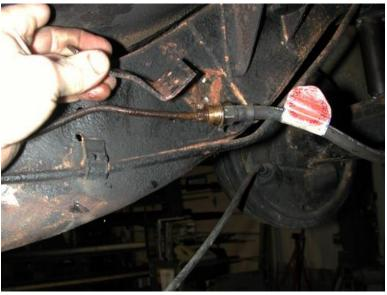
4. The rear brake line bracket on the passenger side fame rail must also be removed.
