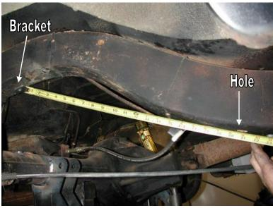
6. The location of the upper Shockwave mount is determined by measuring 20 1/4" from the edge of the bracket to the large hole in the bottom of the frame.
