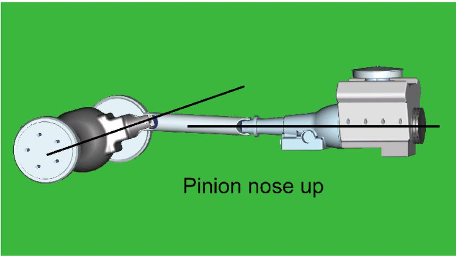
9. How do you set the pinion angle? On a single-piece shaft you want to set it up where a line drawn through the center of the engine crankshaft or output shaft of the transmission and a line drawn through the center of the pinion are parallel to each other but not the same line.
