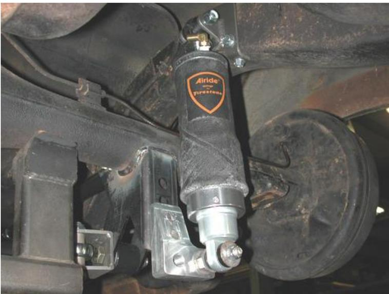
22. Apply thread sealant onto the air fitting and screw it into the top of the shockwave. Air fitting location can be moved by rotating the bellow assembly separate from the shock.
