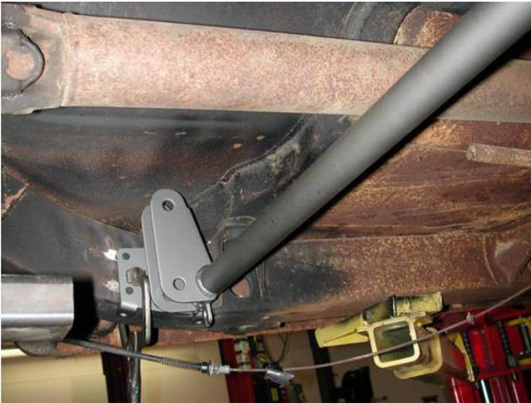
5. Use a couple clamps to secure the crossmember between the frame rails. Slide it forward to the edge of the body mounts. Drill the holes with a 5/16" bit and thread the 3/8" x 1" self-tapping bolts in one at a time.
