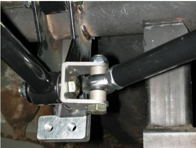
19. Bolt the diagonal link into place with a spacer on both sides of it using a  $\frac{5}{8}$ " x  $2\frac{3}{4}$ " bolt and nyloc. It should measure  $30\frac{1}{4}$ " C-C.
