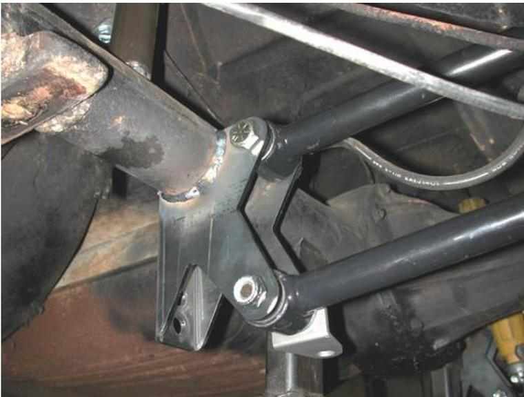
13. Install the 4 link bars into the crossmember and axle bracket, but **do not tighten the bolts yet**. Use the 5/8" x 2 3/4" bolts and nylocs supplied. Check the length of the bars; they should be 18 1/2" C-C.
