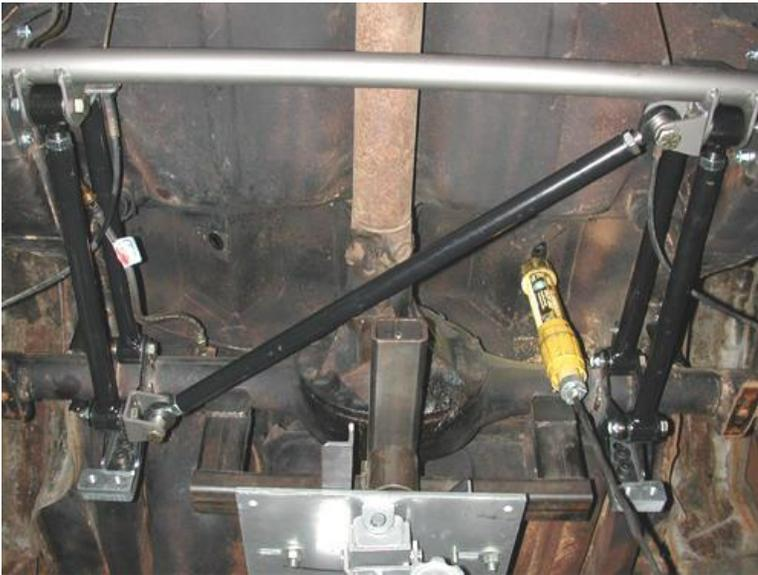
17. Bolt the lower Shockwave mount to the axle bracket using the  $\frac{1}{2}$ "-20" x  $\frac{3}{4}$ " Hex Head Bolt. Apply anti-seize to the threads. It is easier to remove the bars to install these bolts.
