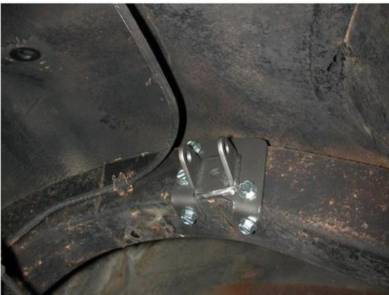
7. Use a clamp to hold the bracket against the inside of the frame and drill the holes with a 5/16" bit. Thread a 3/8" x 1" self-tapping bolt into the frame after drilling each hole.
