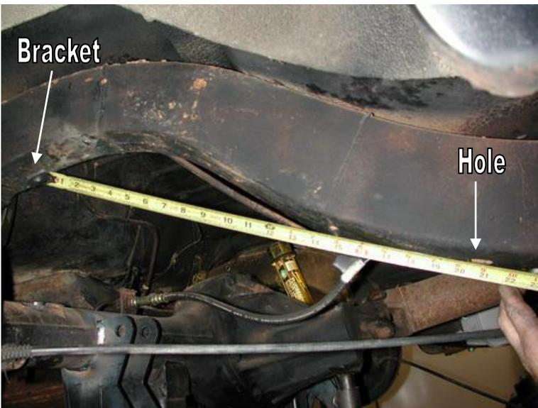
6. The location of the upper Shockwave mount is determined by measuring 14 1/2" from the edge of the bracket to the large hole in the bottom of the frame.
