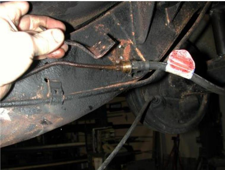
4. The rear brake line bracket on the passenger side frame rail must also be removed. Be careful not to cut fuel line.
