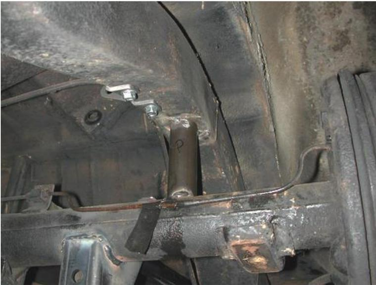
10. Pinion angle must be set at ride height. At ride height there should be 4 1/2" between the axle and frame.
