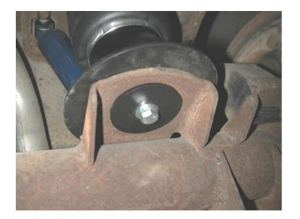
7. Replace the factory shocks with the new ones supplied.
