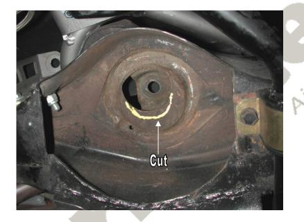
2. The Shockwave stud top will come in contact with the coil spring retainer, so it must be opened up towards the engine. A die grinder works well here.
