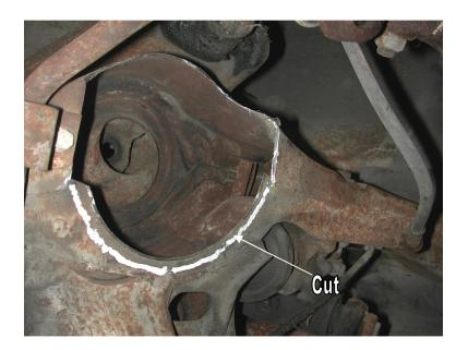
1. To allow clearance for the Shockwave, some trimming must be done on the inside of the coil spring pocket as shown by the white line in the picture. This is best done with either a cut off wheel or plasma cutter. Grind all cuts smooth when finished.
