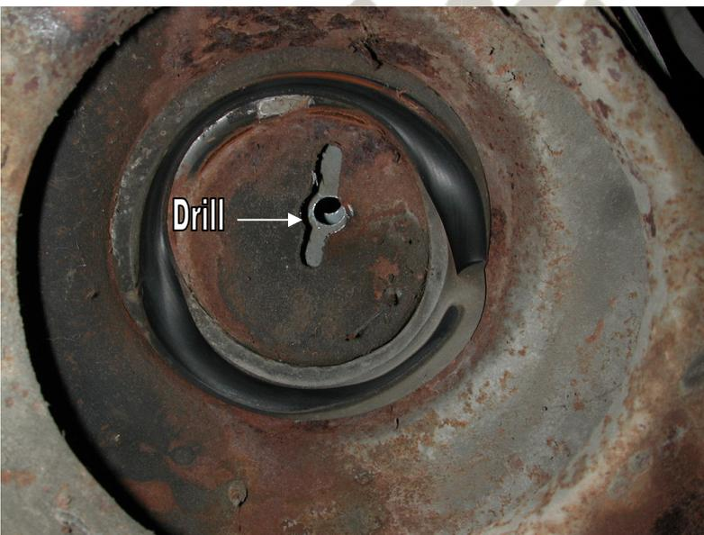
4. You must also drill a 7/16" hole in the top of the coil spring pocket. Use the hole in the center of the slot as a guide.
