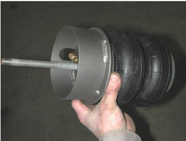
8. Apply thread sealant to the air fitting and screw it into the top of the air spring.
