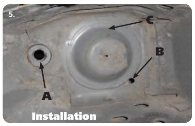
**5.** Picture "5" shows the factory upper coilspring pocket in the car. (A) is the factory shock hole that the upper plate and mounting bracket will be bolted through, (B) is a locating hole in the body that will be used to help locate the new upper plate, (C) is the factory coilpring locator that will also help in locating the upper plate
