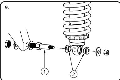
**9.** Drill the factory shock stud hole out to 5/8", this can be done using a Unibit. Install the (1) Shock stud (90001617) into the factory lower mount using the hardware supplied with the stud. Install a 5/8" I.D. spacer on the shock stud, then the bottom of the ShockWave on the stud, followed be another 5/8" I.D. spacer. Install 7/16" washer and Nylok nut.
