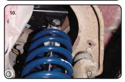
Tighten the lower Coilspring Adjusting nut until the Coilspring is sitting snuggly on the CoilOver. Using the Spanner wrench add another 1/2" of preload in the spring by threading the adjuster nut up the Shock Body. Be sure that the locking screw is lightly tightened in the adjuster nut. Once you have preloaded tighten the locking screw. It may be necessary to add more preload, this will be determined once the car is setting on the ground.
