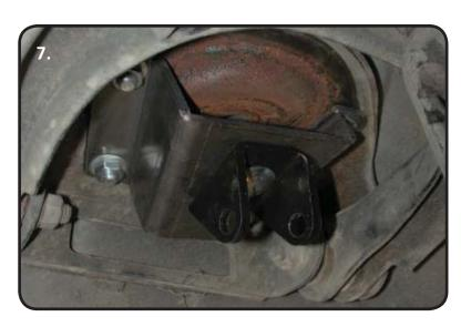
7. Using the 1/2" Carriage Bolt, 1/2" Flatwasher, and 1/2" Nylok, bolt the Upper Shock Mount to the upper bracket. The squares in the brackets should be aligned with the square shank on the carriage bolt. With the squares aligned tighten the mount. With the 2 pieces bolted together, bolt them into the car using (4) 3/8"-16 x 1 1/4", (8) 3/8" Flatwashers, and (4) 3/8" Nylok nuts. There is Driver and Passenger Bracket and this have a "D" and "P" stamped in them. Tighten all hardware.
