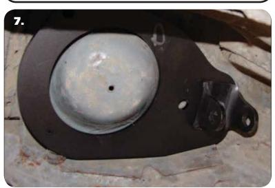
7. Tighten the 7/16" Nut and bolt with the help of the second person. When tightening be sure the upper mount is clocked in a manner that the upper CoilOver mounting bolt will be in line with the lower stud.
