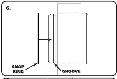
**1.** Install the R-Joint Housing into the OEM bushing hole, making sure it goes in straight. Next, install the supplied Snap Ring into the groove on the bushing housing.
