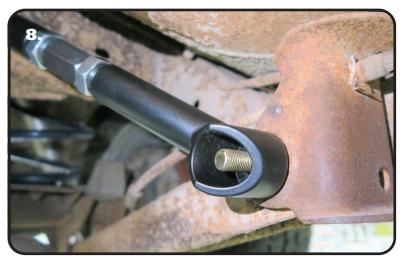
**8.** Install a 1/2" SAE flat washer on a 1/2"-20 x 4 1/2" bolt. Insert the bolt/washer through the OEM brace, lower control arm, and frame brace.
