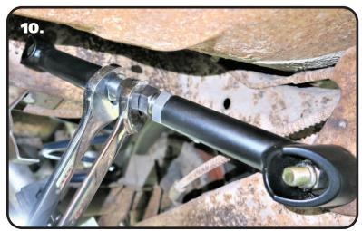
**10.** Tighten the jam nuts against the brace bars.
