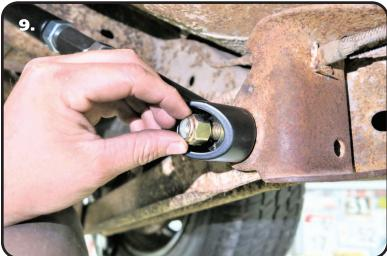
**9.** Install a 1/2" SAE flat washer and 1/2"-20 nylok nut on the threads of the bolt.
