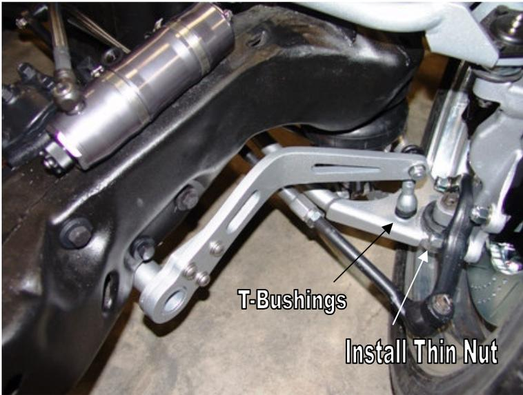
7. Bolt the sway bar arm to the bar using 3/8" x 1" Button head screws with flat washers and lock washers.
