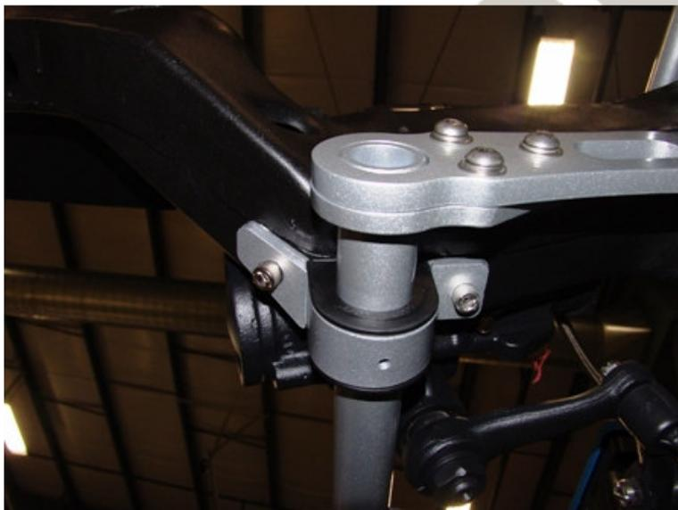
5. Slide the poly bushing over the bar and lubricate with the lithium grease supplied.
