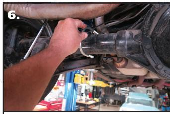
**6.** Install the U-bolts onto the axle tube with the threads pointing down. You may need to raise the brake lines in the area of the u-bolts. The u-bolts will be approximately 23 1/2" apart and equal distance on each side from the brake backing plates.
