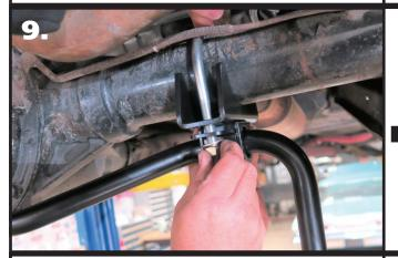
**9.** Hold the SwayBar in position on the car with the center bend toward the ground. Install a 7/16" Flat Washer & 7/16"-20 Nylok Nut on the threads of the u-bolts. Snug the hardware down and verify that it is centered and the axle mounts are level. Torque the u-bolt hardware.
