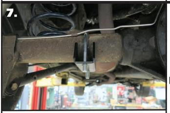
**7.** Install an Axle bracket onto each u-bolt with the flat side to toward the ground. The "teeth" of the mount should touch the axle tube.
